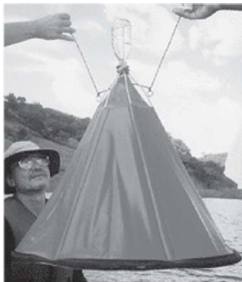
Funnel Bubble Collector Coupled to a Gas Collecting Bottle
